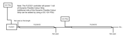
Note: Up to 10 x 5M rolls of FLEX01D can be run from the FLEX21 controller.
