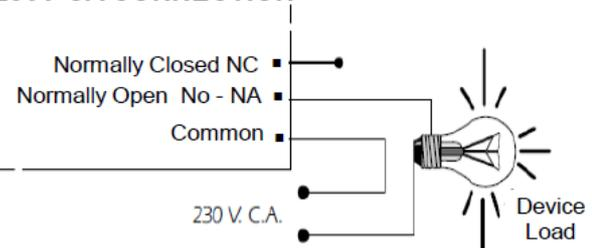
**INFORMATION ABOUT THE OUTPUT.** During the operating mode and according to its load, it could happen a fluctuation or an incorrect working of the output. In such case, you have to install an anti-spark circuit between both contacts of the used relay, as it is indicated on the schedule
