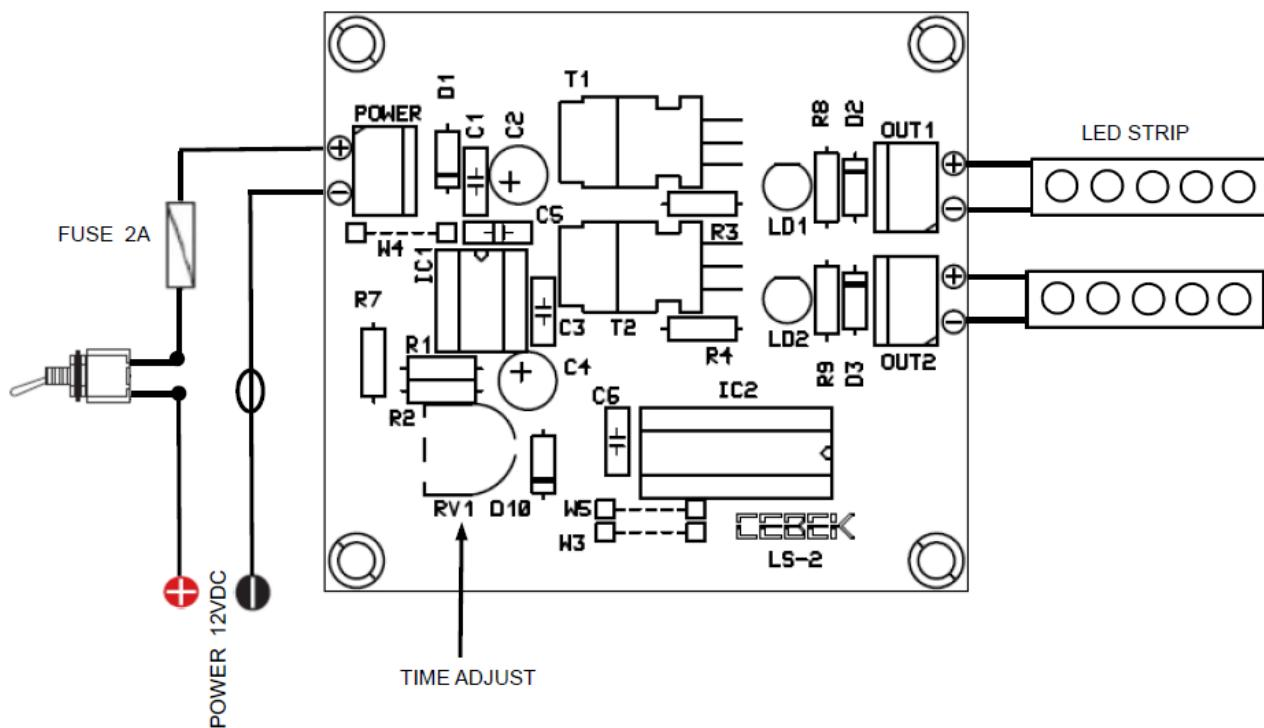
**The LED strips have polarity. Respect positive and negative**
