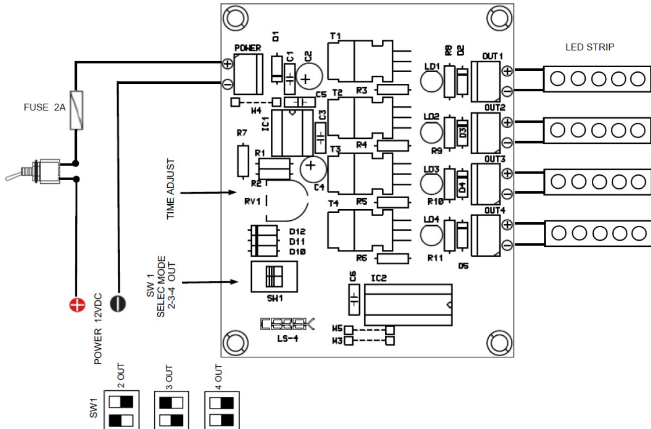
**The LED strips have polarity. Respect positive and negative**
