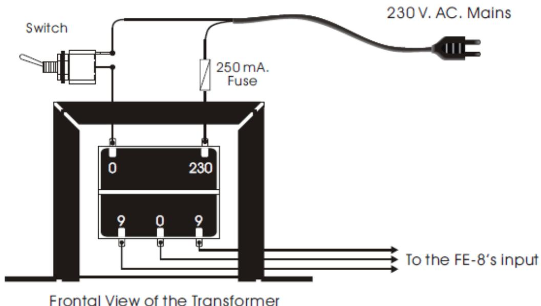
**MODULE'S CONNECTION.** Once the transformer's connection done, you have to verify that the module is not supplied by 230 V A.C. Connect three inferior terminals to the input module's terminals (9, 0 & 9) as it is indicated in the General Wiring Map. Activate the switch and Leds will light indicating that the module is operating.
