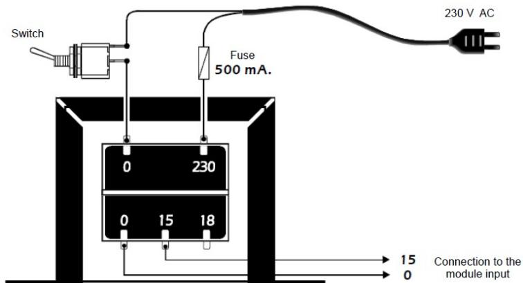
**CIRCUIT CONNECTION.** Once you have connected transformer, connect the circuit.
