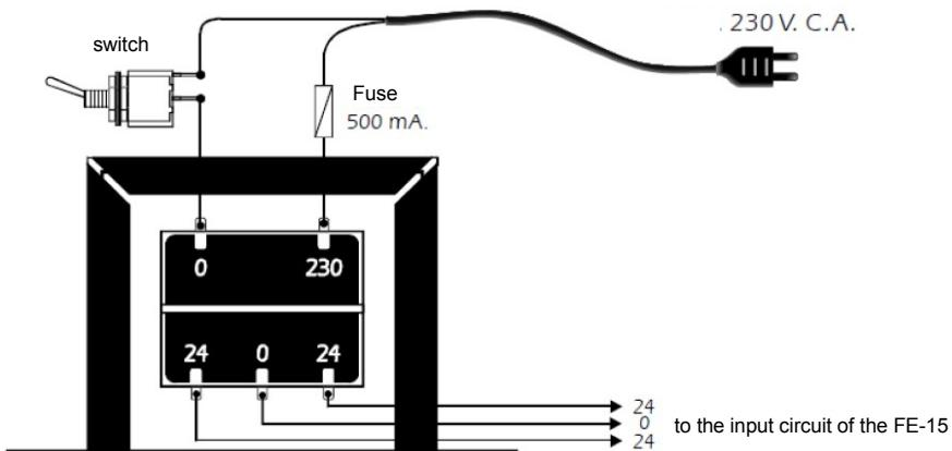
**MODULE WIRING.** Once you have connected the transformer connecting the circuit.
