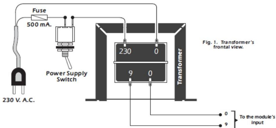
**MODULE WIRING.** Once you have made the connection of the circuit transformer .
