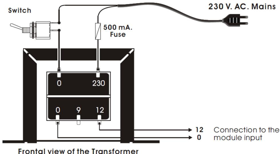
**MODULE WIRING.** Once the transformer's wiring done, you have to wire the module. Firstly, you have to check that there is no voltage (230 V AC) in the module.
