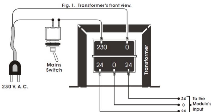
**MODULE WIRING.** Connexion to the three lower terminals of the transformer with the inscriptions "24", "0" and "24" to the input terminal to the circuit.
