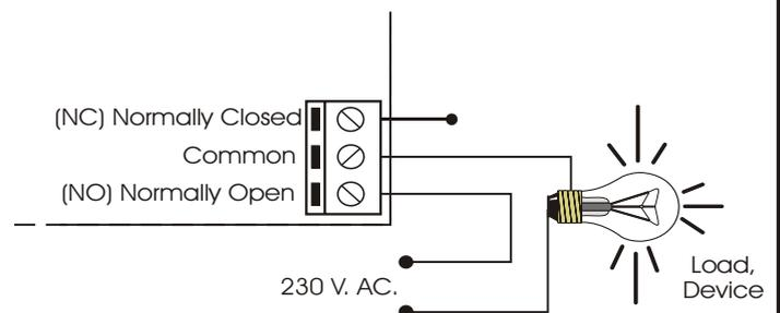
and Common to control the apparatus supply (allowing or stopping the voltage). For the inverse function you have to use the NO and Common. In the drawing hereafter, you could see a typical connection with a 12 V D.C and 230 V A.C devices.
