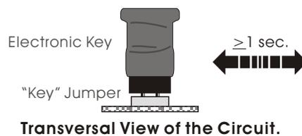
**3rd. Step.** Remove the electronic key from the Key Jumper.
