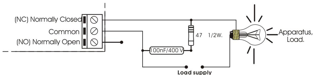
**INFORMATION ABOUT THE OUTPUT.** During the operating mode and according to its load, it could happen a fluctuation or an incorrect working of the output. In such case, you have to install an anti-spark circuit between both contacts of the used relay, as it is indicated on the schedule.
