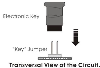
**2nd. Step.** Maintain the electronic key on the Key Jumper during 1 sec. as minimum.
