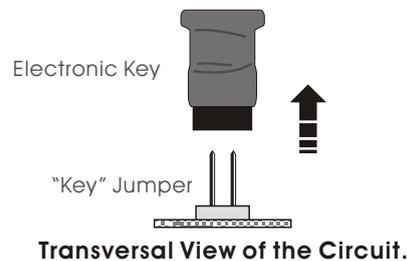
When you insert the key into the key jumper, the status led will completely light on during 2 sec. then, the module immediately start from the beginning the pre-selected timing. Do not forget that each time you "charge" the module, it will start form the beginning the timing.
