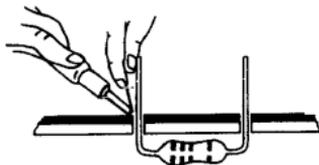
Make sure the solder joints are cone-shaped and shiny
