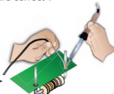
2. Make sure the solder joints are cone-shaped and shiny. →
