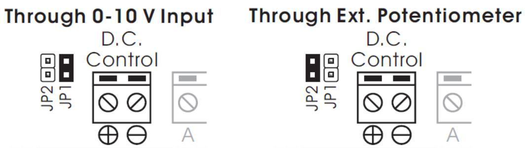
**0-10V SIGNAL INPUT MODE.** If you have placed the Jumper in JP1 position, the module will be configured to adjust the output according to an external input signal from 0 to 10 V DC.
