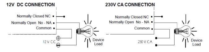
**ABOUT THE OUTPUT :** During operation of the circuit, and according to its load, it could happen fluctuation or an incorrect output performance. If this happens, install a circuit sparking between the two relay contacts used in this connection, as shown in the drawing.
