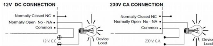
**INFORMATION ABOUT THE OUTPUT.** During the operating mode and according to its load, it could happen a fluctuation or an incorrect working of the output. In such case, you have to install an anti-spark circuit (100 nF/400V Capacitor type X2 and 47 . ½ W resistor) between both contacts of the used relay, as it is indicated on the drawing.
