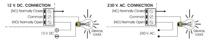
**INFORMATION ABOUT THE OUTPUT:** During the operating mode and according to its load, it could happen a fluctuation or an incorrect working of the output. In such case, you have to install an anti-spark circuit between both contacts of the used relay, as it is indicated on the schedule.
