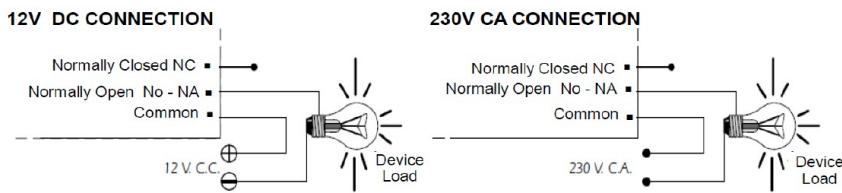
**CONSIDERATIONS ON RELAY:** Especially with inductive loads, a relay output can produce a fluctuation, apportionment, or malfunction. If this happens, install an anti-spark between the two relay contacts used in this connection, that ensure absorption peak current that causes the circuit above problem.
