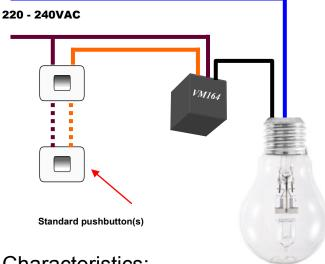
"This mini dimmer fits easily into your existing electrical wiring. Just put in series and add one or more pushbuttons and you are set"
