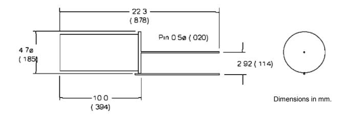
**NOTE:** When cutting the terminals of the sensor, care must be taken not to damage the glass that closes the metal housing. The terminal should not be cut away
