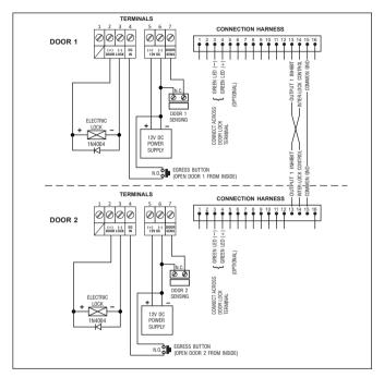
An inter-lock system needs two door controllers. This application example uses two DK-9523 with simple cross wire connection on their "Output 1 INHIBIT" and "Inter-lock Control Output" terminals. It is necessary to link up the "(-) GND" terminals of the two keypads as common ground to achieve the inter-lock logical functions. The connection of the Green LED is optional. It lights up for lock energized.
