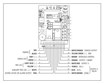
The connection facilities consist one set of terminal block mainly for Output 1 for door lock open; and one set of wire harness for Output 2 and 3, and the auxiliary functions.
