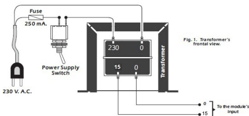
**CIRCUIT CONNECTION.** Once you have connected transformer, connect the circuit.
