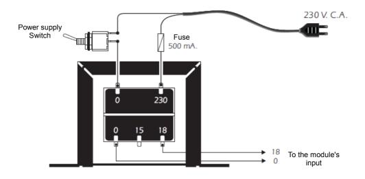
**MODULE WIRING.** Once the transformer's wiring done, you have to wire the module. Firstly, you have to check that there is no voltage (230 V AC) in the module.
