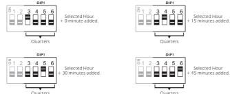
In order to better understand the timing adjustment, we communicate you two samples:
