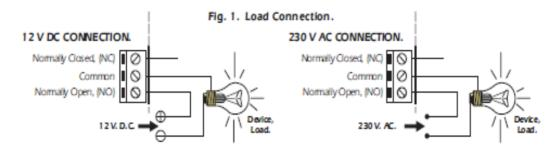
**INFORMATION ABOUT THE OUTPUT.** During the operating mode and according to its load, it could happen a fluctuation or an incorrect working o fthe output. In such case, you have to install an anti-spark circui tbetween both contacts of the used relay. If the load connected to the relay is supplied by 230V, you have to use a 100nF/400V Capacitor and a 47W. ½ W resistor, as it is indicated on the drawing herewith.
