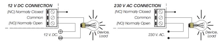
**INFORMATION ABOUT THE OUTPUT.** During the operating mode and according to its load, it could happen a fluctuation or an incorrect working of the output. In such case, you have to install an anti-spark circuit between both contacts of the relay used in this connection, as it is indicated on the drawing.
