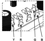
Make sure to put a 1A T (slow-blow) fuse in series with the primary winding
