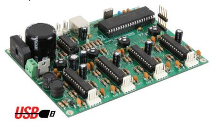
USB controlled stepper motor card, to drive 4 stepper motors. While the motor turns you can simultaneously check the status of the dry-inputs (ex. emergency stop signal, limit detection...).
