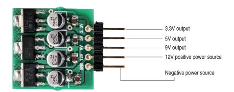
From the circuit diagram, it is possible to see that the three regulators are connected in a parallel configuration, that is to say that the input of each one of them is in parallel with the other ones; thus all three are powered by the voltage applied between the 12 V and GND (ground) contacts. All the contacts (inputs and outputs) are placed on the borders for an easier wiring, and are repeated on a line of spacing 2.54 mm bonding pads, that enables the assembling of a pin-strip.
