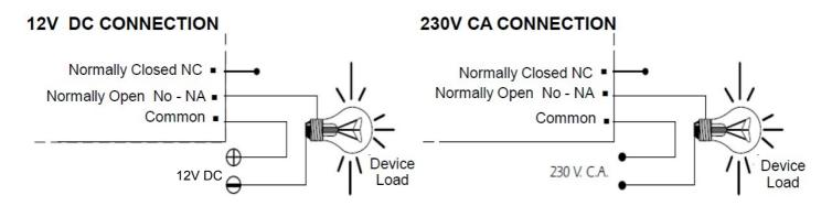
**CONSIDERATIONS ON THE RELAY.** Especially with inductive loads, a relay output can produce a fluctuation rate, or an incorrect operation. If this happens, install anti-spark circuit between the two relay contacts used in the connection, which will ensure the absorption of peak current that causes the above problem.
