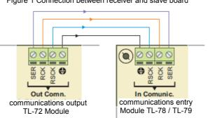
Figure 1 Connection between receiver and slave board
