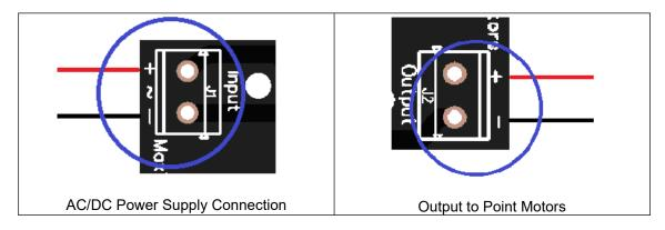
Connect two wires to the output terminals, + should go to the centre pin of the toggle switch and – terminal is connected to the coils of your point motor. Wires should be connected from either side of the toggle switch to the point motor. This can be repeated for other switches and point motors you want to control.
