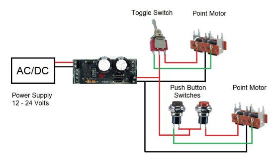
Wiring the CDU is very straightforward. Connect your AC power supply to the input terminals marked  $\sim$  (These can be connected on either terminal). If you are using a DC power supply connect to the same terminals (these are marked + and -). They must be connected the right way or the unit will not function.\*
