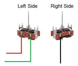
With all the switches in the off position, switch on the power, the LED on the CDU will illuminate. The unit is now ready for operation, when operating one of the point motor switches it will discharge the capacitors in to the coil of that point motor causing the points blades to move.
