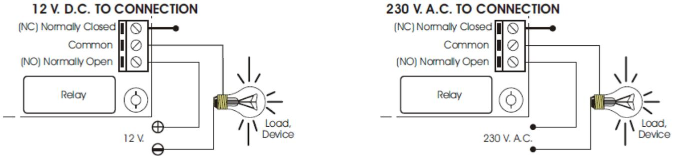
**CONSIDERATION TO THE OUTPUT. LOAD.** During to the operating the module according to be charge, you can happen the fluctuation or incorrect output fonctionament. This is wrong you have install the anti-spark (resistor & capacitor), between two contacts of the relay make's in the connection such as is to apper in the
