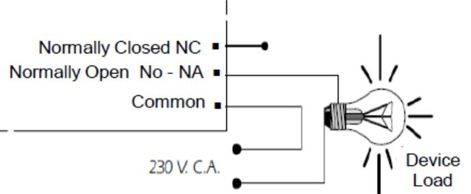
**CONSIDERATIONS ON THE OUTPUT.** During the operating mode and according to its load, may fluctuate or malfunction departure. If this happens, install a circuit spark between the two relay contacts used in connection as shown in the drawing.
