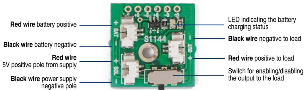
The charging current ( $I_{reg}$ ) is set by the resistance connected to pin 5 (R1 in our case). The current value is reckoned as follows:
